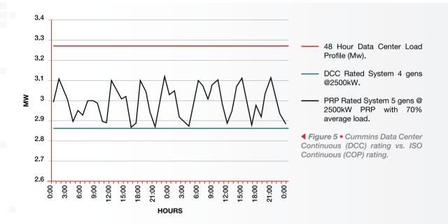
This light load is very common in real-world data centers. As the graph shows, the COP rated generators are running below 30 percent of their maximum horsepower, while the DCC rated generators are running above 30 percent of their maximum horsepower. The DCC rated generator system is the more reliable choice in this example, and it will operate closer to the optimum horsepower of the engines, reducing the risk of low load failures.
