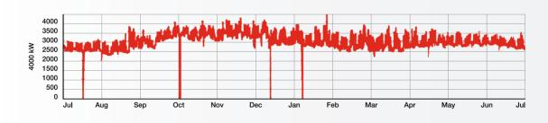
**Figure 3 •** Typical data center load profile.
